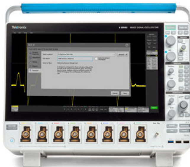
Figure 5: Save a session to TekDrive just like any other drive on the oscilloscope
