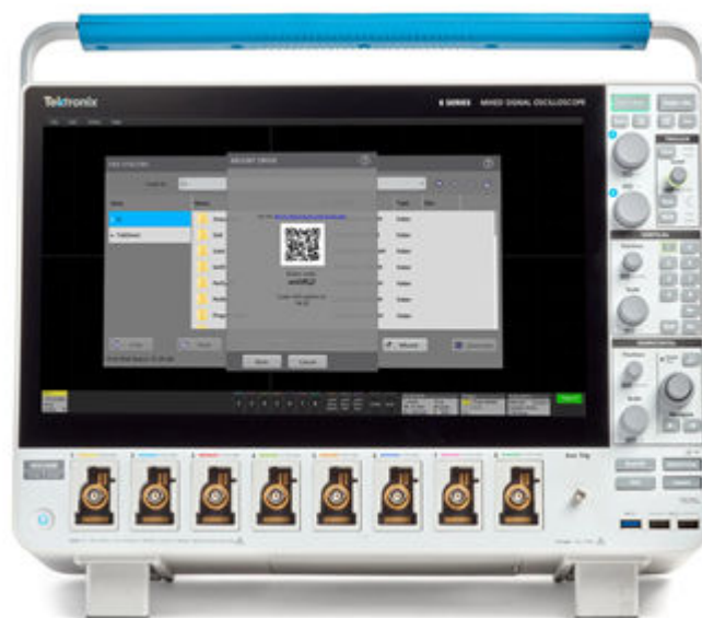
Figure 4: Mount the TekDrive on an oscilloscope using a short-code style login system.
