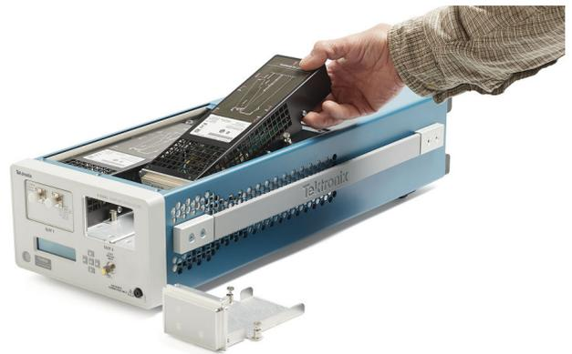
Plugging TSO8C18 module into TSO820 mainframe.
