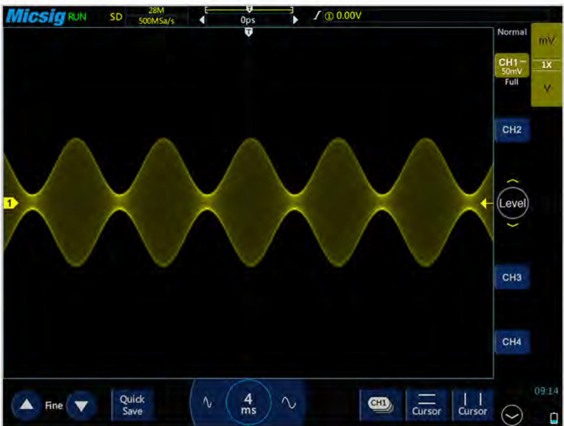
Gradient waveform display with 256 intensity levels
