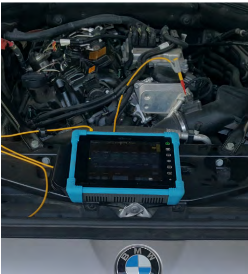
BMW Air flow meter test
