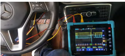
Power CAN bus communication
