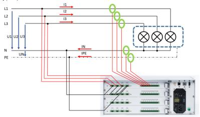
It is recommended, but not necessary to use fuses of type 500mA for the voltage connections.
