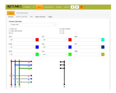
Connect the instrument as shown in the following picture (connection may vary with different board types):
