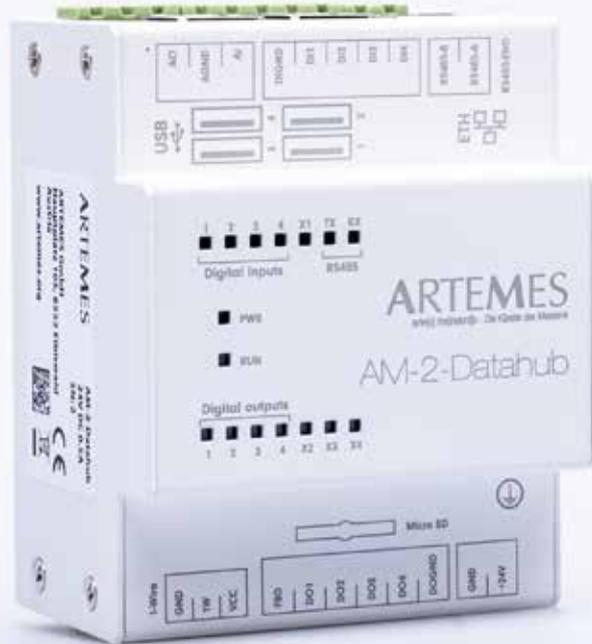
The AM-2-Datahub in the space-saving DIN rail housing is **the perfect communication tool** in the family of ARTEMES' measurement and monitoring solutions which is able to connect various components.
