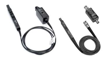
The P6021 and P6022 Current Probes provide versatile AC current measurements. Both probes provide accurate current measurements over a wide range of frequencies. The P6021 and P6022 allow current measurements without breaking the circuit by clipping onto the current carrying conductor. Shielded probe heads are not grounded when the slides are in their open positions, eliminating accidental grounding of the circuit under test.
